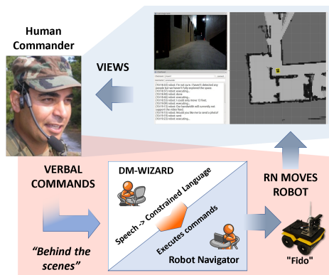
Figure 1: WoZ Experiment Setup, where a CMD gives vocal instruction to a remote robot, represented by the two-wizard setup
